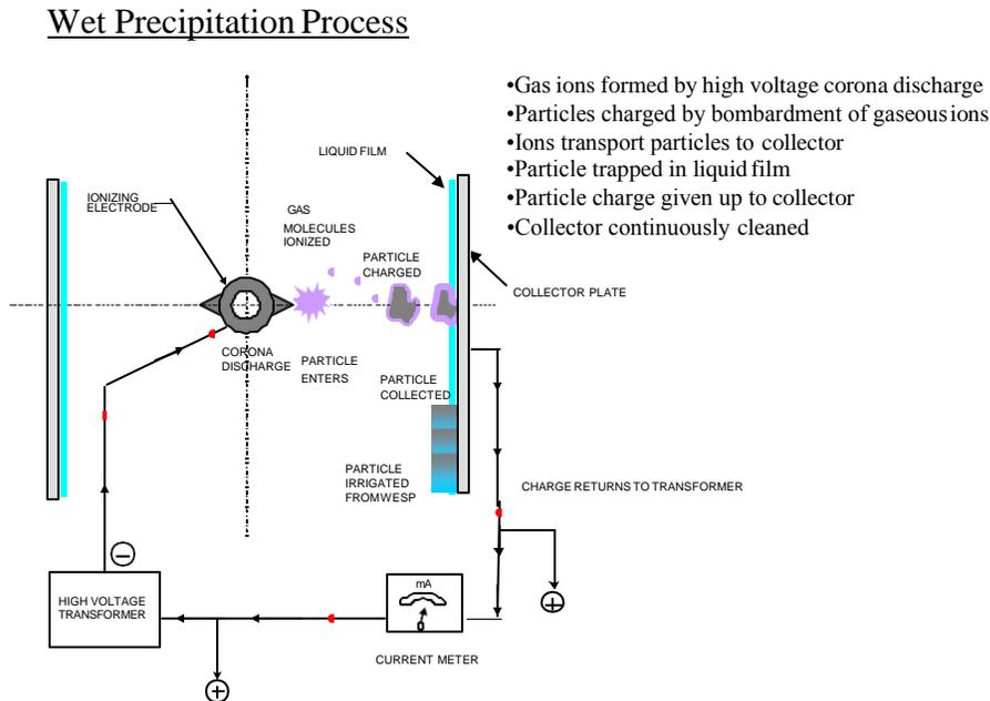
While the cleaning mechanism would not be thought to have any impact upon performance, it significantly affects the nature of the particles that can be captured, the performance efficiencies that can be achieved and the design parameters and operating maintenance of the equipment. Simply stated, wet ESP technology is significantly different than dry ESP technology.
