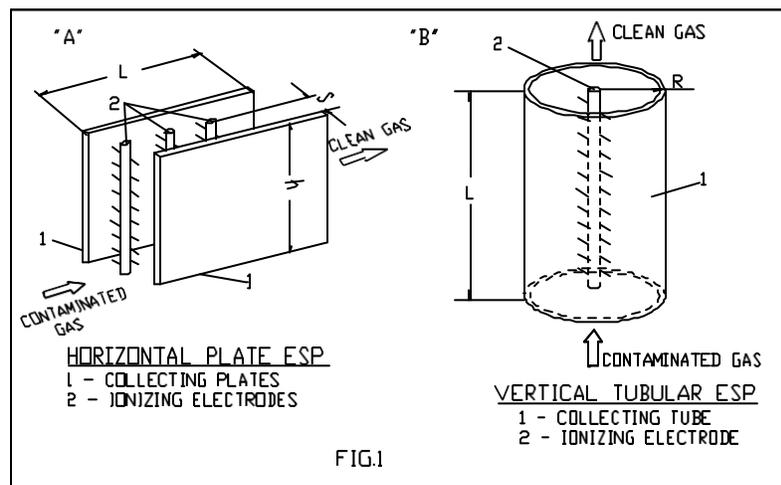
Figure1: The comparison of a tubular WESP vs. a plate type WESP shows that, for a given efficiency, a tubular WESP can operate at twice the velocity of a plate type WESP, resulting in a smaller footprint (Applicable mostly for new construction).
